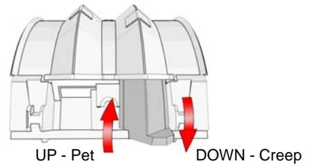
Note: Remove detector assembly as described in Fig. 1. When selector is UP, Pet Mode; when DOWN, Creep Zone is active and there is no Pet Immunity.
