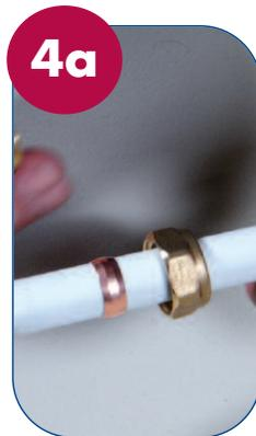
✓ Push the pipe into the compression fitting.
