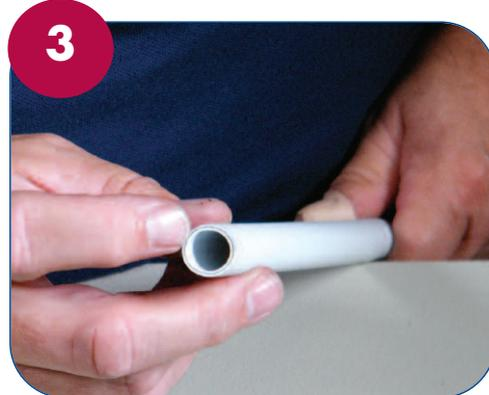
✓ To reduce the risk of leaks, ensure you check the cut pipe is free of imperfections.
