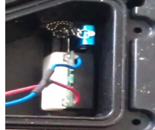
**Step4:**insert another end of Adapter cable to battery
