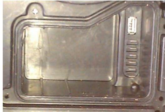
**Step2:** insert the U disk to the USB port
