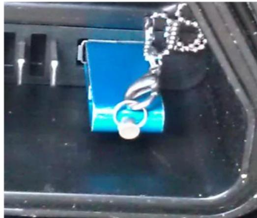
**Step3:**insert one end of Adapter cable to battery connector
